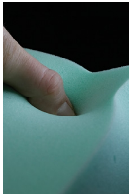
Thermofresh® by Pelma S.p.A. Polyurethane foam embedded with PCM
